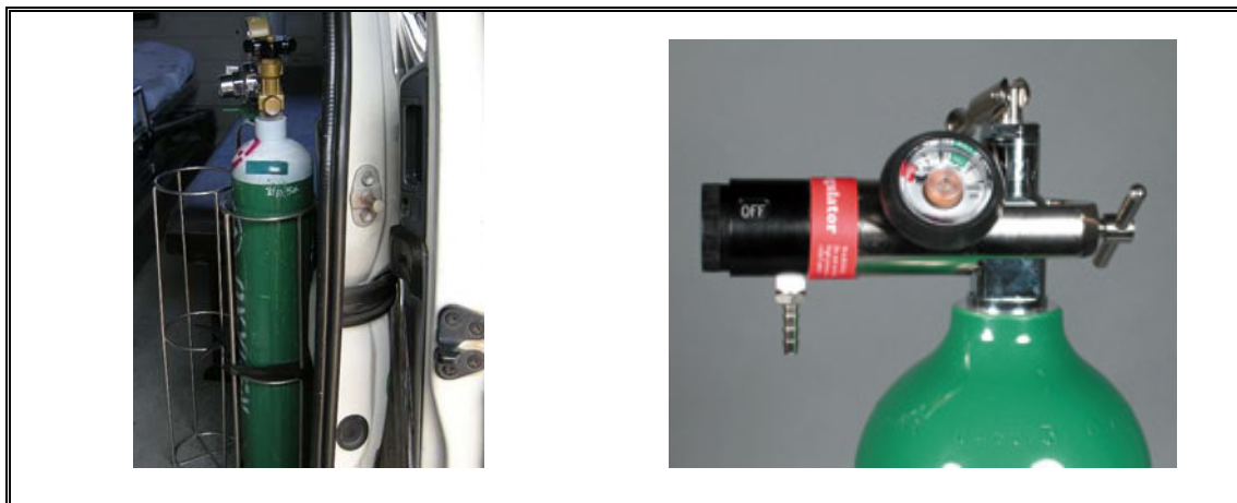
Figure 4: Portable oxygen unit nearly the exit for convenient use with the pressure gauge and flow metre
